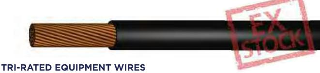
Plain annealed stranded circular copper conductors, circular high temperature PVC outer sheath. UL & CSA approved also to BS6231. 600/1000 volts grade. Flame propagation to BS EN 50265 and IEC 60332-1.
