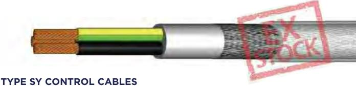
Plain annealed flexible copper conductors, PVC insulated, extruded PVC bedding, galvanised steel wire braid armour, transparent PVC outer sheath. 300/500 volts grade generally to BS6500 and VDE 0250 class 5.
