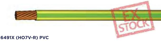
Stranded plain annealed compacted circular copper conductor, PVC outer sheath. Ref 6491X. Harmonised code HO7V-R. 450/750 volts grade to BS EN 50525-2-31. Flame propagation to BS EN 50265.
