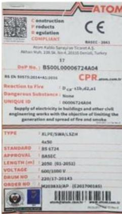
Cleveland Cable Cut Ticket replicates details of the CE label in greater detail
