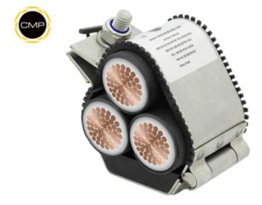
CMP Patriot cable cleats are metallic cable cleats which have been designed, constructed, and tested in accordance with the International Standard IEC 61914: Cable cleats for electrical installations to ensure the securing and retention of cables, without sustaining damage to the cable.
