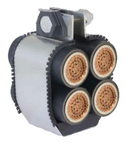
CMP Saturn quad cable cleats are metallic cable cleats which have been designed, constructed, and tested in accordance with the International Standard 'cable cleats for Electrical Installations' IEC 61914 to ensure the securing and retention of cables, without sustaining damage to the cable.
