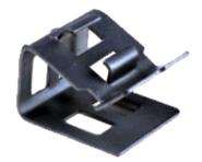
Girder clips offer a quick, easy & reliable method of fixing solutions to steel work, without the need for bracket making, drilling holes or the use of nuts and bolts.
