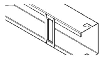
Legrand Steel Trunking - Cable Retainer
